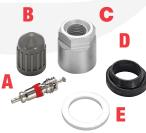
The OEM requires that the valve stem components are replaced every time the tire is serviced on vehicles with TPMS.
